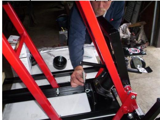
10) Push the lift top down as you guide the neck over the cylinder head (jack) making sure the cylinder head is placed inside the oval collar. Screw up the cylinder head to take up slack between the cylinder and the neck, this gives you maximum height on your lift.
