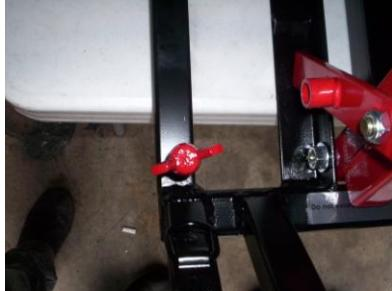
9) Attach the spring to the end of your foot pump first and then to the eye bolt on the lift. Do not over bend the spring, it will weaken and eventually break. There should be a small metal "hook" on the bottom side of the foot pedal to attach the spring to.
