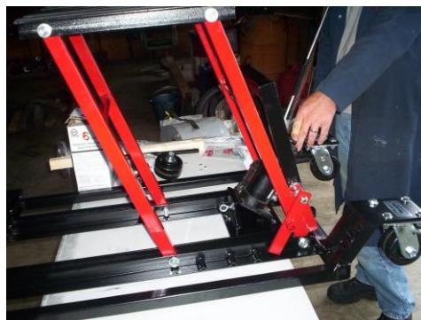
4) Hydraulic model only: Take the set screw out of the collar on the jack cylinder that your foot pump handle goes through and install your foot pump handle. Place the set screw back into the collar, do not over tighten.
